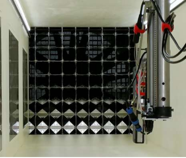
Figure 2: Experimental setup: The 8 \times 8 axis active grid installed in the Environmental Wind Tunnel at WUT.
